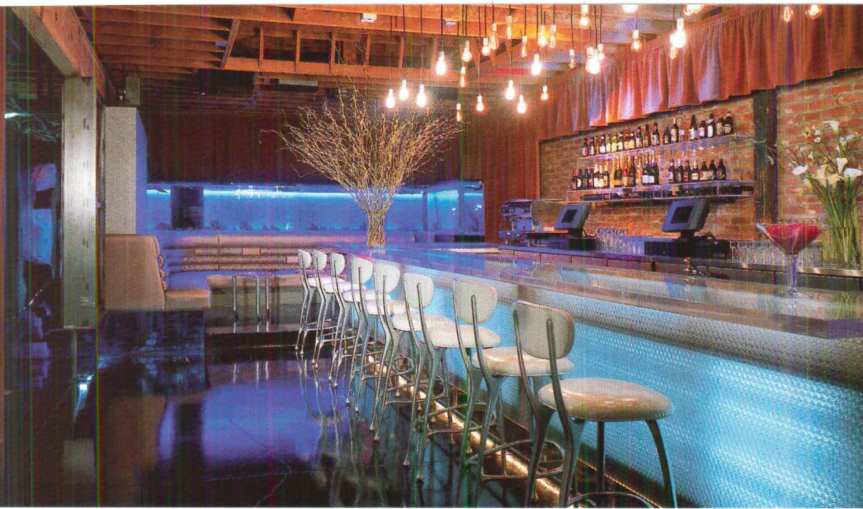
Acrylic abounds in the honeycomb sheeting over the bar front (left) and the two-inch-thick clear slab above it. Restroom doors are also clear acrylic (below), offering views to the lavatories.
