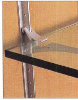
"ellen's brackets", an anodized-aluminum shelving system designed by M Ali Tayar, provides an elegant alternative to existing bracket-and-track systems. Cantilevered brackets come in two sizes, for shelves 3/4 or 3/8-in. thick and 10-in. deep. Wall-mounted tracks permit 1 1/2-in. adjustment of wood, glass or plexiglass shelves. For more info phone Parallel Design Tel: 212/989-4959 Fax: 212/989-4977.
