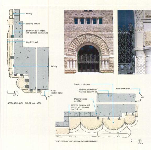
**H. H. Richardson** might have disapproved, but the massive-looking stone arches and walls of Hale Library are hand-laid stone veneer anchored to poured-in-place concrete backup walls. Kent Bloomer's maquettes were used by Alan Tollackson in hand-carving the trim for the building's stone arches. Bloomer also designed and fabricated the metal screen that spans the arch.
