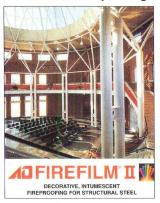
Improved spray characteristics and ratings up to 3 hours! A/D FIRE-FILM®II permits designers to use the appearance of exposed steel with the steel protected from fire. The product is applied as a thin-film coating 0.4 to 3.3 mm (16 to 130 mils) thick. When exposed to fire it expands to form a meringue-like insulating layer up to 4 in. thick. A/D COLORCOAT topcoat is available in a wide range of colours. Call 1-800-263-4087 or 416-263-4087. Internet: www.adfire.com. See us in Sweets.
