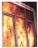
Pemko Mfg. Co. introduces FireGlaze™ (FG3000), a specially formulated high performance glazing compound. This revolutionary product allows for the use of much larger vision lites, side lites, borrowed lites, and glass transoms in 20, 45 and 90 minute doors and screens. The "wall of glass" pictured here passed a 45 minute fire test! Expand your vision.
