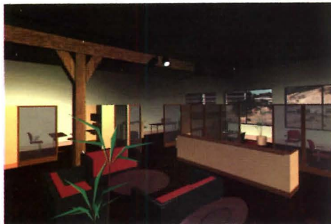
The wireless-frame image (1) grew out of a 2-D AutoCAD floor plan. It was rendered in 3-D Studio and saved in Adobe Photoshop to produce image at right (2). Note the video-captured landscape through the windows in the more detailed closeup above (3).
