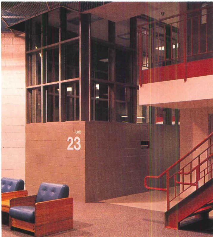
Between 36 and 40 cells ring each 1,200-square-foot dayroom (above). While an officer is stationed at a desk in the dayroom (left in photo above), he is supplemented by an officer in a control booth (below) who oversees two sets of housing units.
