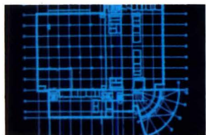
Structural grids created automatically.
