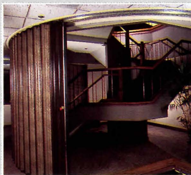
Code Required Occupancy Separation without compromising the appearance of an elegant stairway or other design feature.
