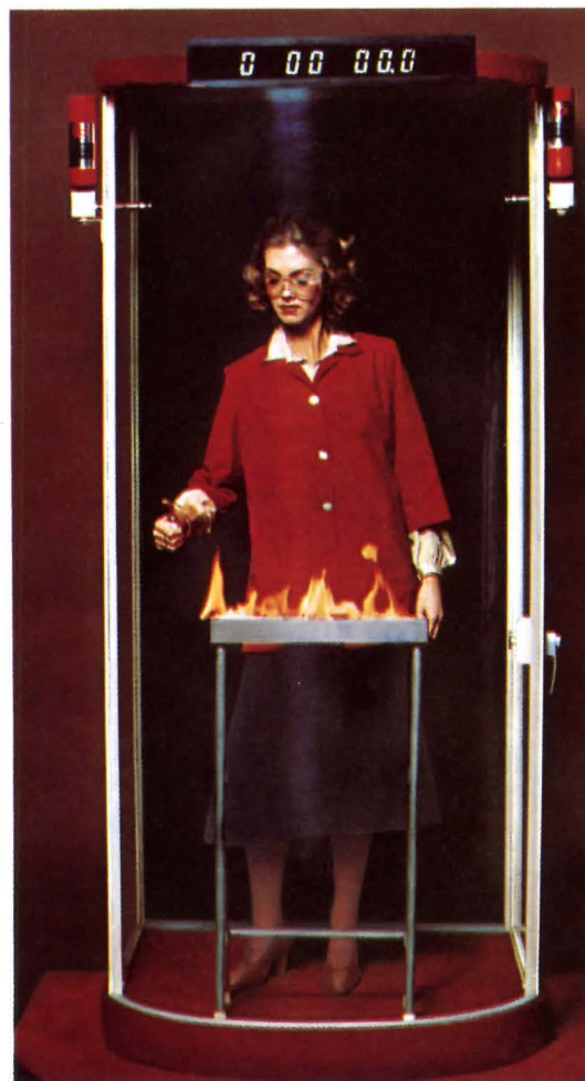
1. Flammable liquid ignited. Halon 1301 cylinders discharged.
