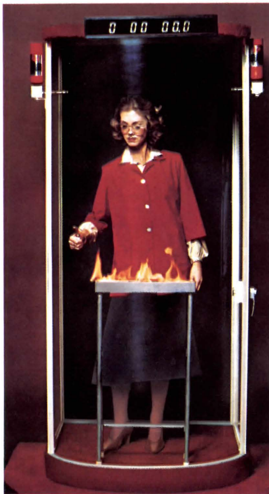
1. Flammable liquid ignited. Halon 1301 cylinders discharged.
