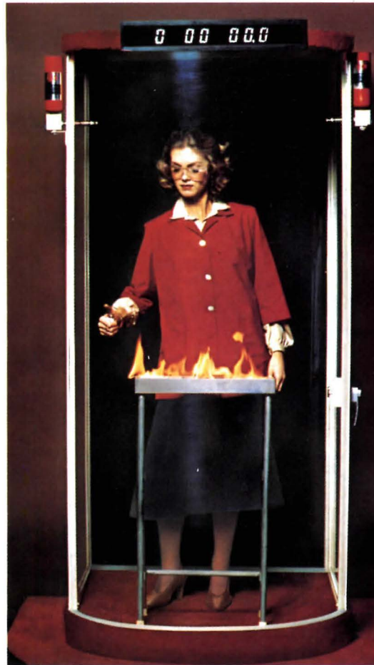
1. Flammable liquid ignited. Halon 1301 cylinders discharged.
