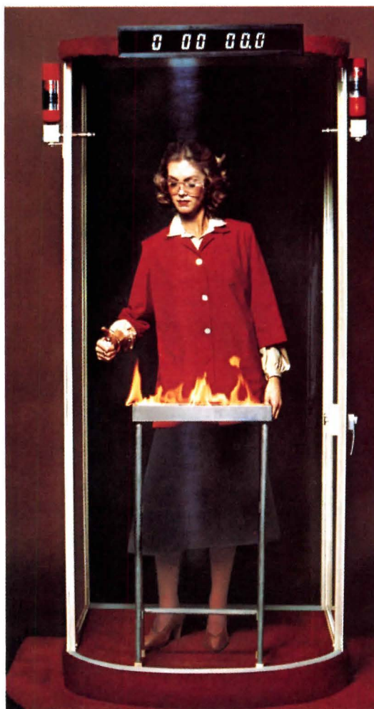
1. Flammable liquid ignited. Halon 1301 cylinders discharged.
