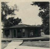
CIRCULAR BUILDING / Prefinished Carousel modular structure has clear span roof and walls. Insulated walls, insulating windows and doors. Sizes to 2580 sq ft, for slab or pole foundation. / Distinctive Homes Inc.
