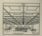
Exclusive with American Louver-Paracube louvers in 3'x3' size for large area luminaires and luminous ceilings designed for 3'x3' modules. Other sizes 2'x2', 1'x4', 2'x4' for all applications.
