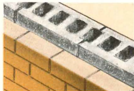
2 For non-aligning horizontal joints.
