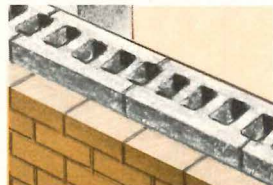
3 Cavity walls restrained in the horizontal span.
