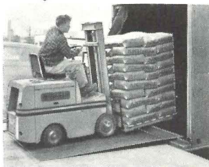
Torsion bar actuated hinged lip dock leveler
