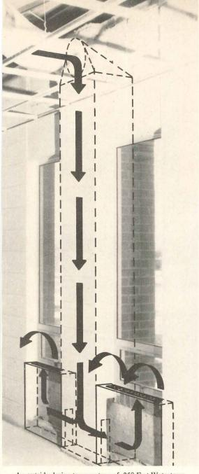
An outside design temperature of -25° F at Watertown, South Dakota, made it desirable to have perimeter distribution of heat in the Watertown Vocational-Technical School. This was achieved by ducting some 20% of supply air down pilasters into wall ducts. Balance of air was supplied by ceiling ducts. Architects: Harold Spitznagel & Associates; Pope and Robel. Engineer: Harold Spitznagel & Associates.
