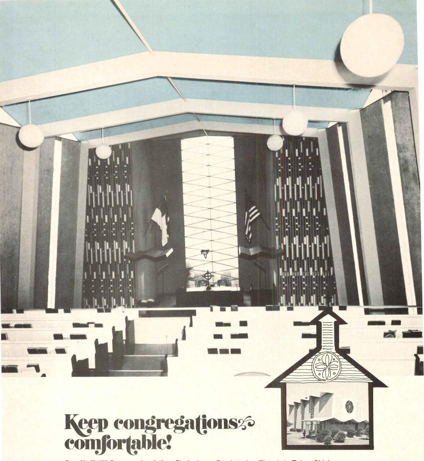
Specify K-13® Spray-on Insulation. St. Andrews Presbyterian Church in Tulsa, Oklahoma, eliminated condensation and solved acoustics problems with a ¾ inch thick application of K-13 on the 4 inch concrete slab ceiling.
