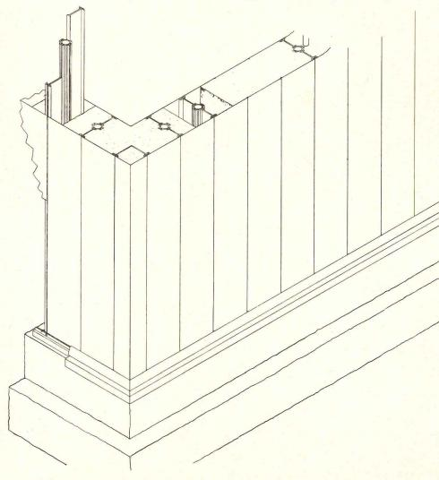
with the wall panels and the use of a metal ceiling and a metal roof deck. The steel inner faces of the panels are attached by clips to the steel frame, and for grounding purposes are bonded by welds at 2-ft intervals. The aluminum outer faces are, of course, isolated electrically from the inner steel panels because the vinyl connectors are non-conductive.
