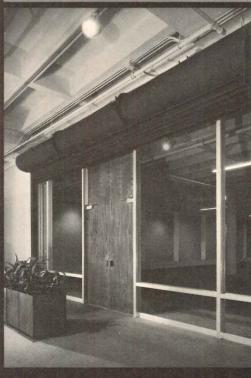
Out-of-the-way not only because Cookson "Servire" Fire Doors and Counter Fire Doors are engineered to save space and present an attractive appearance, but also because they provide a number of special protection features. Included is a fully automatic drop mechanism—with an adjustable governor to regulate the speed of descent—instantly activated by a link that fuses at 165 degrees F.
