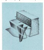
EPICORE makes it go up faster, easier and at less cost. EPICORE offers the industry's strongest most flexible hanging system for ceilings, lighting, piping and other utilities. The inverted triangular ribs key into
