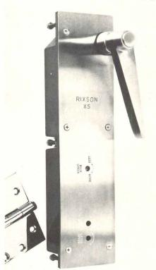
**DOOR CLOSER** / The *X-5* concealed floortype interior door closer has been "designed in response to an extensive survey of architects." It can be removed without removing the door. It can be used with stock hollow metal, aluminum or wood doors and frames with standard 4½-in. by 4½-in. butt hinges, may also be hung on offset or center pivots, and will fit in a two-in. slab. The closer is recommended for mediumtraffic interior doors weighing up to 200 lbs. ■ Rixson Inc., Franklin Park, III.
