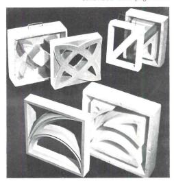
**CEMENT BLOCKS** / A new method of producing cement blocks uses polystyrene forms molded to the desired shape. After the concrete is poured and cured, the block is shipped to the building site in its mold, reducing breakage. ■ Durable Cement Corporation, Chicago.
