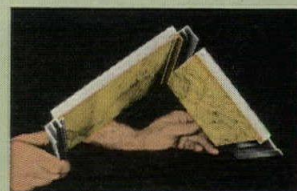
A water tight triple barrier wall connection is formed by the slotted side wall panel as it engages the aluminum extrusion attached to each side of the back wall. Requires no caulking or sealant. Note matching corner molding that makes cleaning easy.
