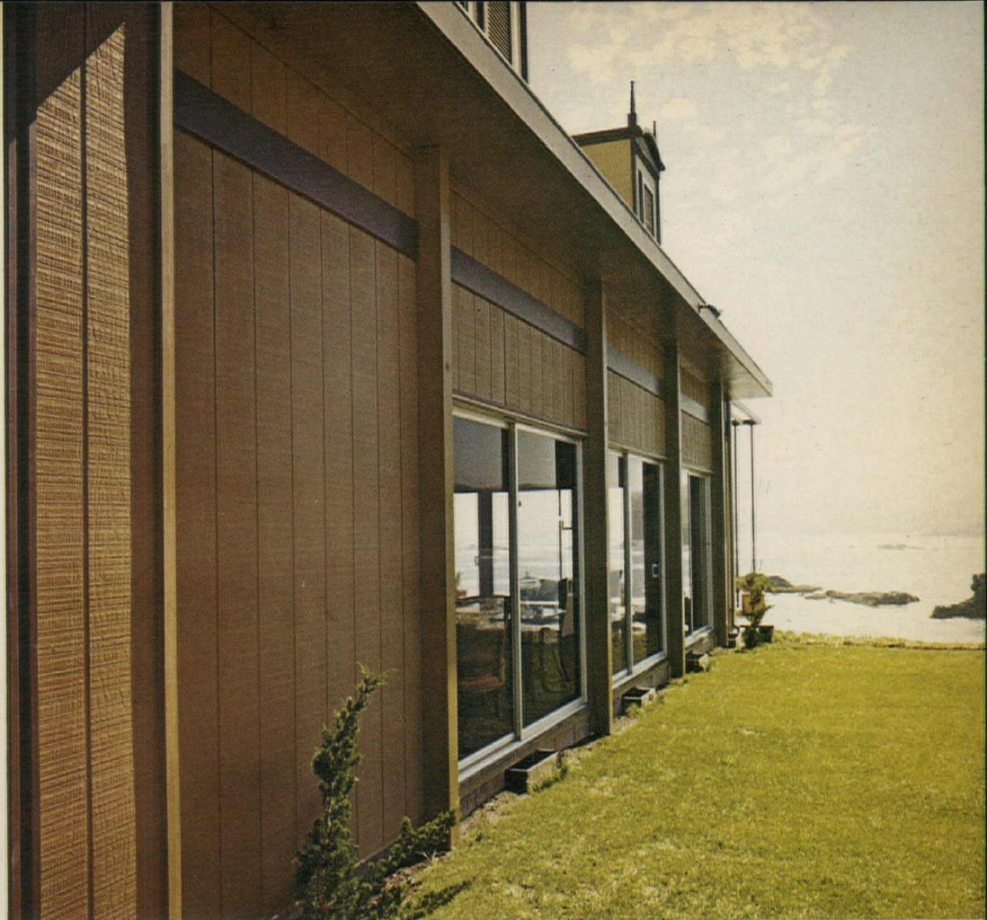
RUF-X-90 Panelgroove siding , ½" square cut grooves on 8" centers, 4' wide; 7', 8' and 9' lengths. Rough-sawn textured finish—factory primed. Also available with ½" V-grooves on 5½" centers.
