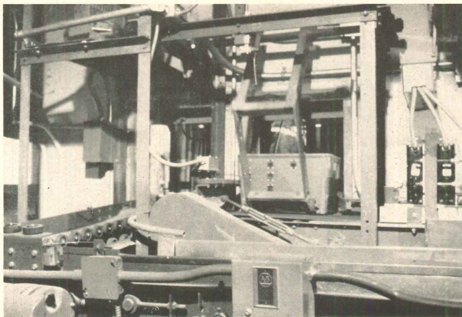
A tray being swept into the vertical conveyor after traveling on a horizontal conveyor from the main sorting area at a rate of between 120 and 150 ft per minute.
