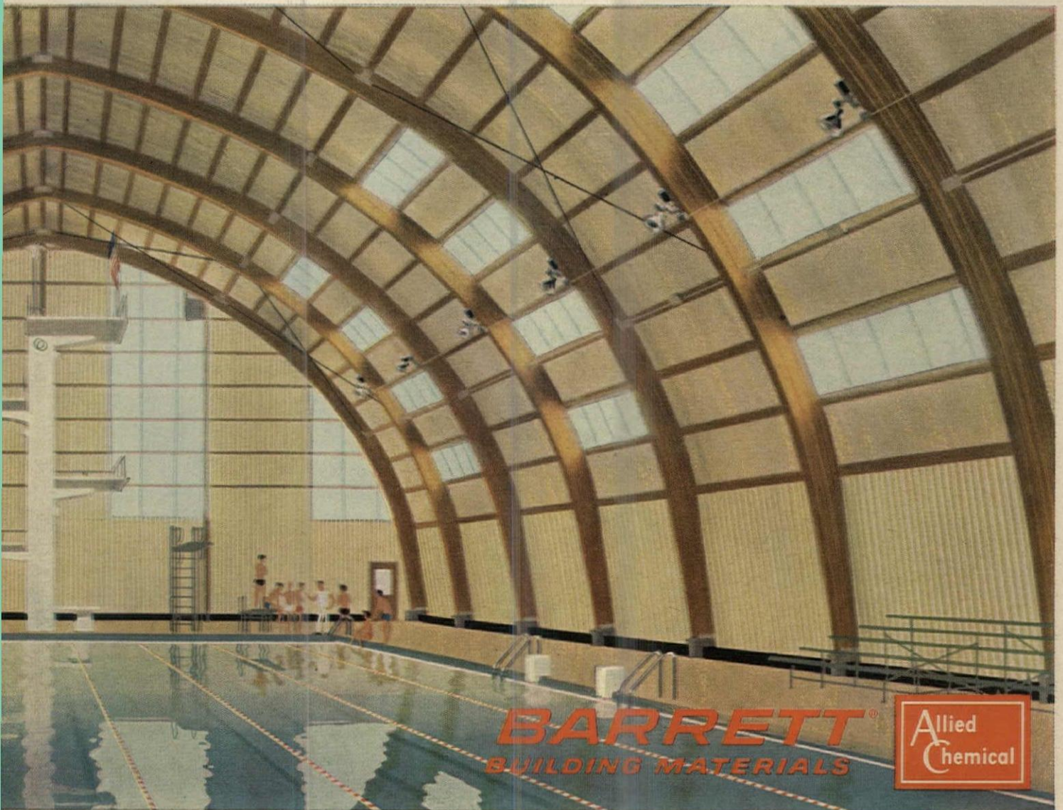
Three 48' sections of flexible 8 oz. Barrett Vinyl Panels were used to make each complete arch over the Philadelphia Aquatic School. This structure is 90' x 197' x 46' 6" high. Exterior steel cables anchor vinyl panels to building's frame.
