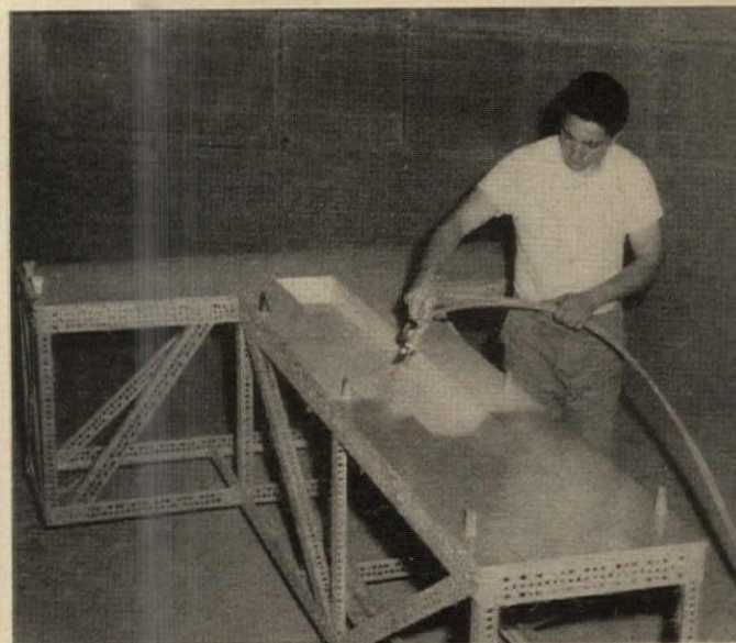
A plastic gel undercoat, which gives the form its extremely smooth finish, is sprayed into the female mold
