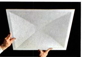
are moulded entirely of fiber glass with an NRC of .75. They are 24" x 24", rising gently to create a 2" vault. As you see above, the surface is made more visually interesting by a low-relief, rippled texture. White-painted at the factory for easy repainting if desired, Textured Vault Panels offer an opportunity to create a sense of height and elegance, as in the gallery above, and in larger institutional or commercial building areas.
