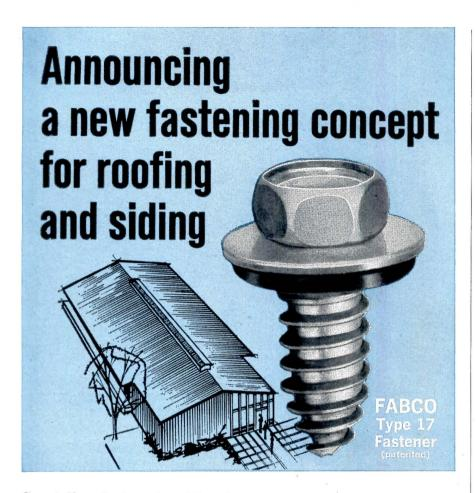
Specially designed with close-clinching threads, special tapered point and standard ¾" hex head, this new fastener is used for: 1. Fastening sheet side laps. 2. Attaching sheets to light gage structural framing. 3. Fastening flashing to sheets. 4. As plugs, where smaller diameter fasteners have failed.
