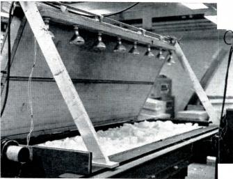
Dry ice, 3 to 4 in. deep, dumped on top of the test specimor drops the temperature of roofing all the way down to -100 F
