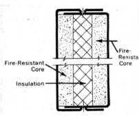
core at both front and back surrounding an interior core of gla fiber. Over-all thickness is  $2\frac{1}{8}$  if Ingram-Richardson Mfg. Co., Beav Falls, Pa.
