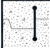
Williams Waterstops are made from Natural Rubber Stock and designed for maximum effectiveness in any type of cast-in-place construction joint. They will bend around corners, and will not crack or tear from shear action. Tensile Test: 3990 lbs., Elongation Test: 650%. Available in rolls up to 80 feet in length. Molded union and junction fittings available. Williams Waterstops can be furnished in Vinyl or Neoprene for industrial uses where resistance to oil or other injurious wastes is desirable.
