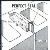
Williams "Perfect-Seal" (Pat. Pend.) is a specially designed seal for use in Mortar-Keyed Control Joints... it provides continuous four-point pressure-contact sealing which keeps moisture out of joints and prevents air passage. The T-Section is a high-grade rubber compound; the cross-sealing member at the base of the "T" is a strip of readily compressible, non-absorbent, expanded closed-cell Neoprene Rubber—it provides an effective pressure-contact seal directly behind the calking.
