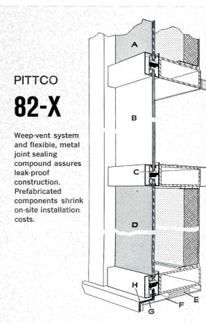
E. Leveling shims F. Flashing
