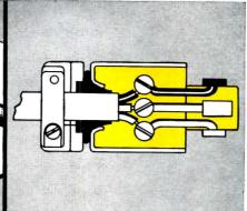
NO AIR SPACES INSIDE PLUG TO COLLECT GAS OR MOISTURE. After plug is wired to cord, electrician pours a self-hardening insulating resin into all air spaces. Interior of plug becomes solid, water-tight, vapor-tight mass.
