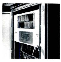
Electronic memory and paging switches in central brain of registry system. "Books" of 100-name printed circuits are added by plug-in
