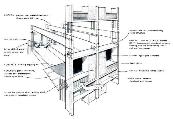
PRECAST CONCRETE STRUCTURAL-MECHANICAL DIAGRAM
