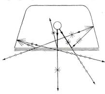
Multi-layer polarizer, enclosure and fluorescent tube. Vertical ray from tube does not become polarized. Other ray directly transmits 45 per cent of its light polarized. Eventually, according to Marks, 71 per cent of this ray becomes polarized by reflection and refraction
