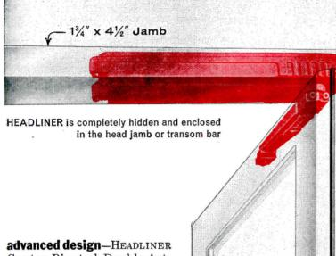
advanced design—HEADLINER Center Pivoted Double Acting Overhead Door Control is built in . . . and performs out of sight, even when doors move to the full-open position. No visible hinges, closers, arms,
