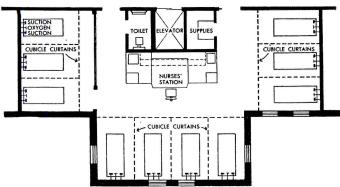
TEN BED INTENSIVE CARE UNIT. Typical Intensive Care unit with ten beds, three of which are separated from main nursing area by partition. The nurses' station is centrally located and a small supply room is provided. Suction and oxygen outlets are provided at each bed. More highly developed versions of Intensive Care units would ordinarily have larger space for storage and an area for consultation
