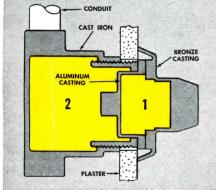
TWO SAFETY CHAMBERS IN WALL OUTLET. Gastight chamber No. 1 (bronze and aluminum castings) contains and seals off switching mechanism. Cast iron chamber No. 2 keeps minor internal explosions from spreading to room.
