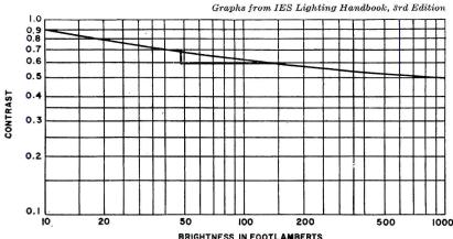
A loss in contrast between an object being viewed (say a pencil mark) and its surround (the paper) must be made up by increased illumination for equivalent no-glare visibility. This chart shows that a reduction in contrast from 0.7 to 0.6 due to glare (14 per cent loss in contrast) is compensated by a 300 per cent increase in brightness of the task
