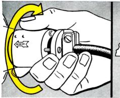
NO ARCING WHEN PLUGGING OR UNPLUGGING. Outlet is electrically "dead" until plug is inserted and rotated 22-25°. Reverse turn disconnects current before plug is removed. Spring pressure and keyed construction prevent accidental disconnection.
