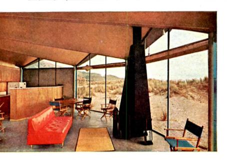
And what a house for enjoying the out-of-doors! Architect Jock McKay designed it with huge window-walls, a sheltered court for sunning, and a unique, "folded-plate" roof. Let the wild winds blow—this house is framed with *steel*. The same design in conventional stud-wall construction would have cost considerably more.
