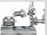
Vertical split-case construction permits easy servicing without breaking pipe connections.
