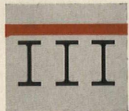
Rigid Wheeling 3/8" Rib Lath transfers loads to joist along strong vertical axis only.
