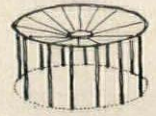
French Pavilion, Zagreb, Yugoslavia, 1935. Single layer of cables; 110-ft diameter, sag/diameter ratio, 1/11. Roof is 14-ga sheet steel hung from steel compression ring. Bernard Lafaille, Engineer
