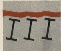
Wheeling's 3/8" Rib Lath doesn't allow load to be transferred along weak horizontal axis . . . thus causing "dominoing."
