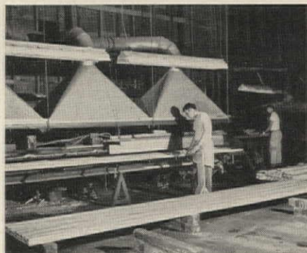
For wide widths, the end-glued pieces are grain matched and edge-glued together.
