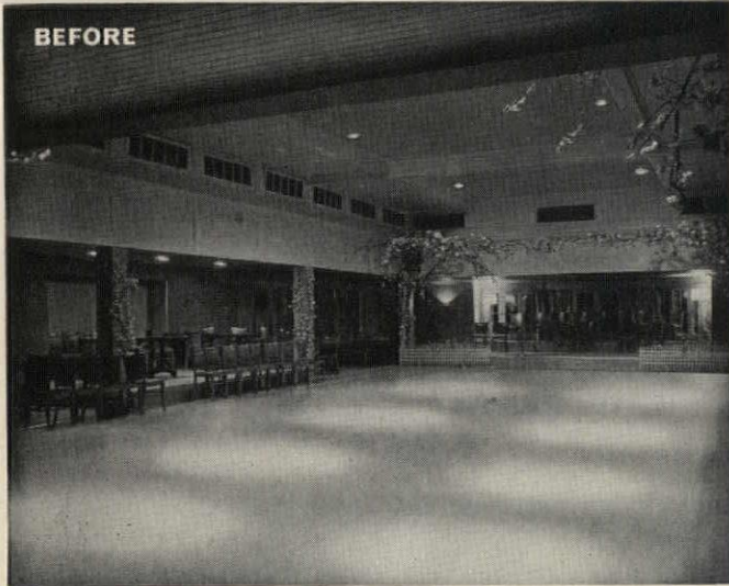
BEFORE DOWN LIGHT - TOO CONCENTRATED Low-brightness on the object you are looking at No brightness on the vertical surfaces
