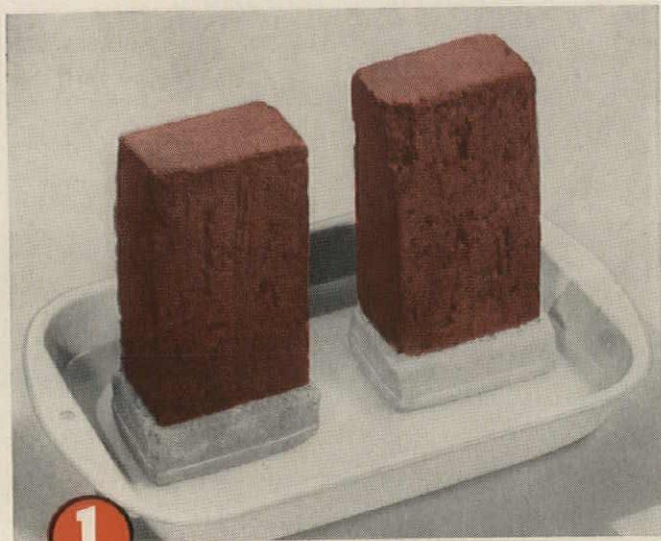
1 Cap one brick with Brixment mortar, about 1" thick—and one brick with ordinary cement-and-lime mortar. After the mortars have hardened, place both brick in a pan of shallow water.
