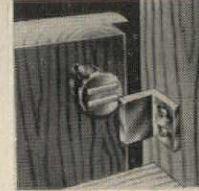
602 Round magnetic catch press fits into 7/8" bore in door. Aluminum case. Self-aligning to enlarged strike.
