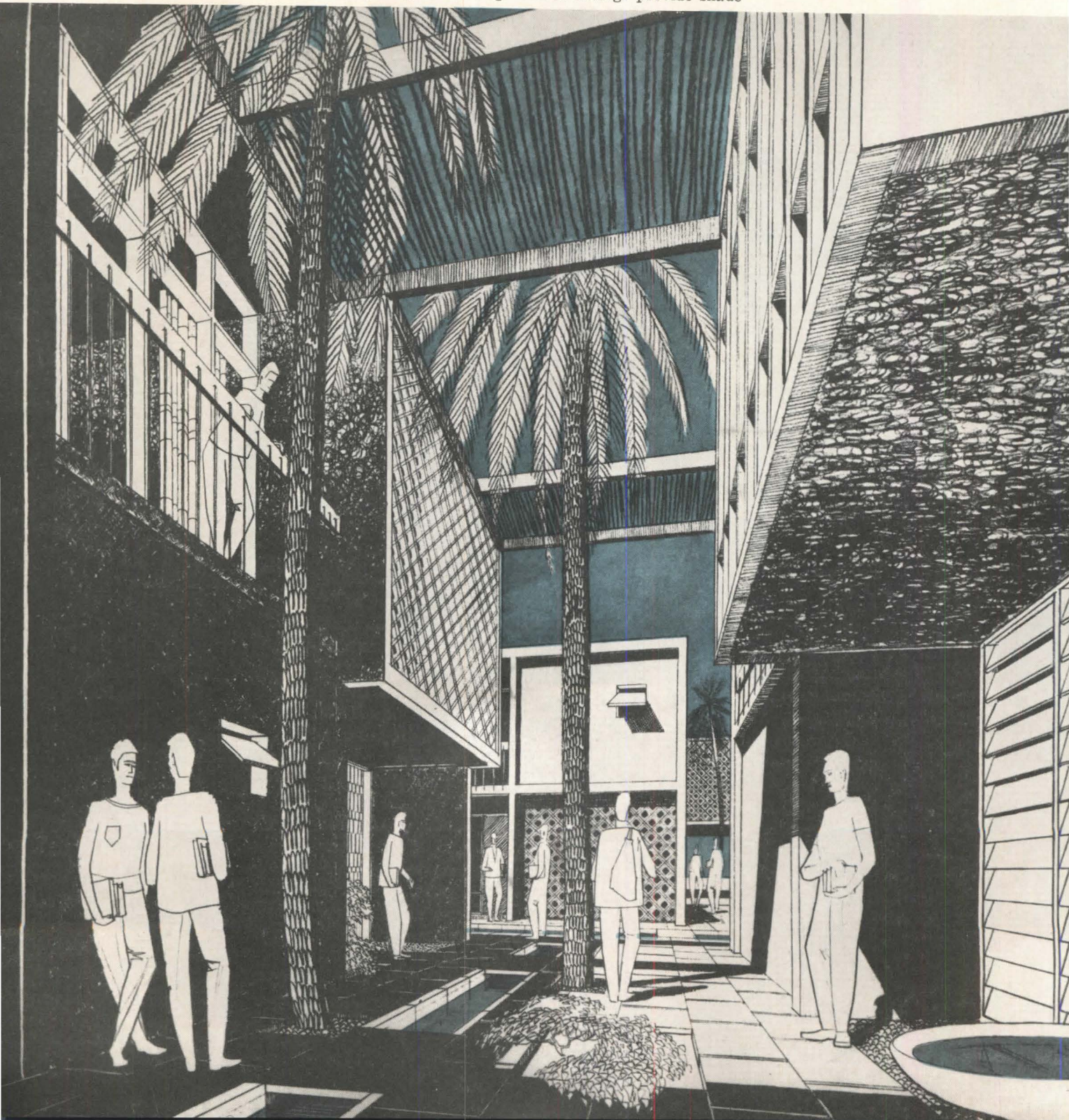
Typical dormitories. Note that close spacing of buildings and overhangs provide shade
