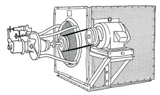
$Figure\ {\it 2.}$  Combination motor-driven and turbine-driven inducer can operate on steam, when power fails
