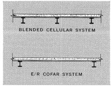
LESS FRAMING. Cofar reinforced concrete construction permits wider spans, saves on structural framing costs, speeds up building completion and permits earlier occupancy by the owner.
