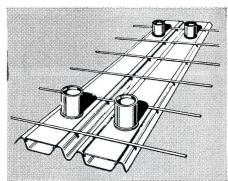
PRE-SET INSERTS. Costly concrete drilling is eliminated by optional pre-set inserts. Install outlets after building is occupied! After-set inserts may also be used with E/R Cofar.
