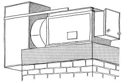
Figure 3. One place for a draft inducer is atop the short chimmy  $% \left( 1\right) =\left( 1\right) +\left( 1\right) +\left$
