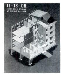
Exploded assembly drawing of the typical apartment building shown above, illustrating manner of joining precast parts
