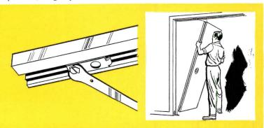
To remove doors, loosen just one nut on top track socket. Slide toward center. Top pivot and guide slip out of track. Just lift door off bottom pivot and away they go for painting, etc. Fastest, simplest removal ever—and from either side!
