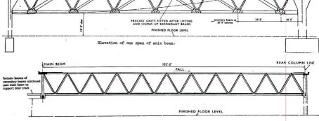
Cross-section of hangar showing side elevation of secondary beam.
