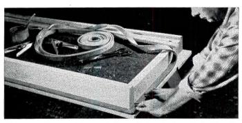
**Tight Seal** is assured by carefully applied gasketing. Gasket is soft sponge rubber resistant to acids, oils and greases.
