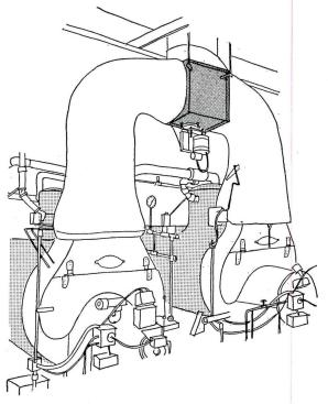
Figure 6. Here one draft inducer in the breeching serves two boilers
