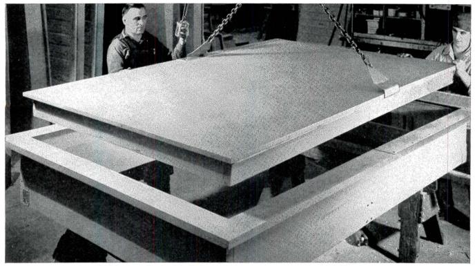
Box girder construction of highest quality boat hull plywood gives maximum strength and rigidity. Large series "50" door is shown as door and frame meet on assembly line.
