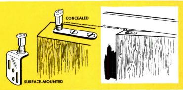
**Doors can't fall out of track.** New suspended guide won't let them — no matter how out of square they may be. Rubber snugger and stop eliminate door play, rattles. Nylon pivots and guides provide really quiet operation, long dependable service.
