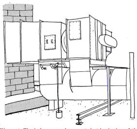
Figure 4. The inducer may be mounted at beginning of the breeching  $% \left( 1\right) =\left( 1\right) \left( 1\right)$
