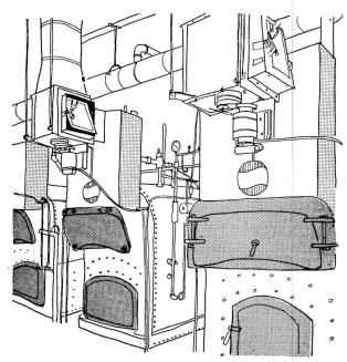
Figure 5. Ceiling suspension is frequently a way of installing inducers in boiler rooms
