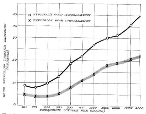
A comparison of the noise isolation effectiveness of a typically poor and that of a typically good installation of folding doors
