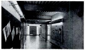
At Northport, a dropped ceiling at the end of the hall conceals mechanical equipment, and heightens the contrast between the uneven light from wood-baffled fluorescents over display boards in the corridor itself and the brightly-lit entrance at the end
