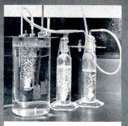
2 Steam condensate corrosion test
