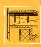
Typical detail and photo of Kalser Aluminum's Type K-1 Gravel Stop. Note simplicity and pleasing shadow line that results from the straight drip edge feature.
