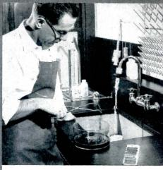
3 Cleaning specimens with inhibited hydrochloric acid
