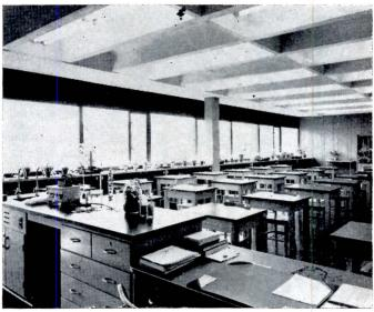
MULTIPLE USE OF STRUCTURAL MATERIAL AND FORM: in the Conard High School, West Hartford, Connecticut, reinforced concrete pan construction enabled exposed structural ceilings throughout for structural, finish, acoustic, and esthetic purposes, and provided builtin light baffles to house inexpensive fixtures. Nichols and Butterfield, Architects
