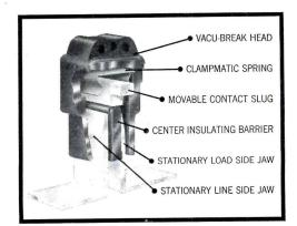
VACU-BREAK CONTROL snuffs arcs immediately when breaking circuits under load. The enclosed head limits the oxygen available during the brief arcing period. Closeness of the head material causes the arc to cool and extinguish quickly. "Double-break" action reduces the distance the Vacu-Break head must travel before the arc is extinguished. In addition, Clampmatic action assures bolt-tight contacts, accelerates breaks.
