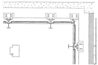
Above: Inside corner detail showing serpentine marble facing. Solid concrete wall is part of wind bracing system. Below: elevation and section of window and spandrel. The section shows the special low profile, high pressure, high velocity air-induction units used on the periphery of the building. They are recessed in the floor construction to achieve an even lower profile.
