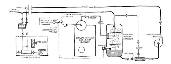
Two-stage, steam-to-high temperature water system showing water level control, high temperature blending and a typical tenant installation
