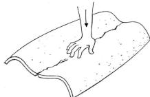
Rupture by bending of a non-compound laminar structure
