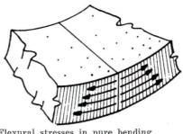
Flexural stresses in pure bending
