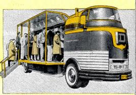
Movable wings open on the sides of the Coaches, exposing exhibits and providing spectator ramps. Special electro-hydraulic system raises brilliantly lighted canopies 8 feet above coachtop level for nighttime displays.
