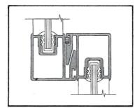
Weathertight integrity, water and dust resistant; a single plane network of Shlegel wool pile weatherseal and cam action of door on closing assures tightest possible seal.
