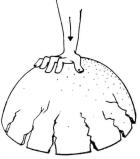
Rupture by tension of a doubly-curved shell
