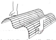
Figure 2: A thin (flexible) cylindrical shell can be maintained in a rather unstable equilibrium as long as its cross-section conforms to the pressure line of the external loads (left). Any slight changes in their distribution or in the shape of the cross-section of the lamina produces rupture by bending due to instability or buckling (right). To prevent this the cylinder must be stiffened by rigid arches or diaphragms
