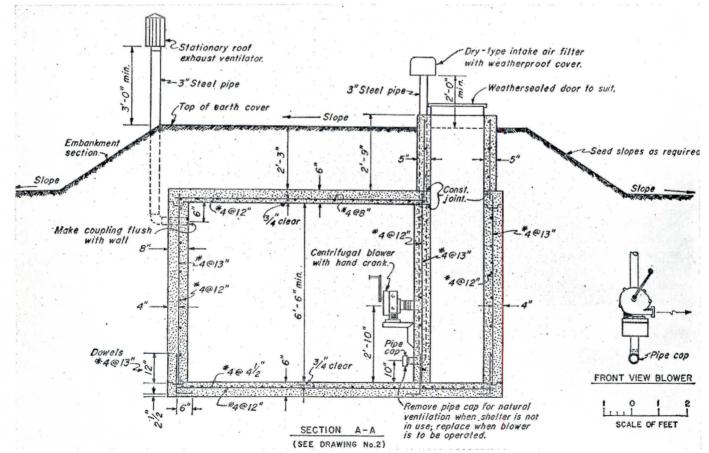
Drawing above (from Civil Defense Technical Bulletin TB-5-3) is longitudinal section of "basic underground family fallout shelter"—described as a "reinforced concrete
