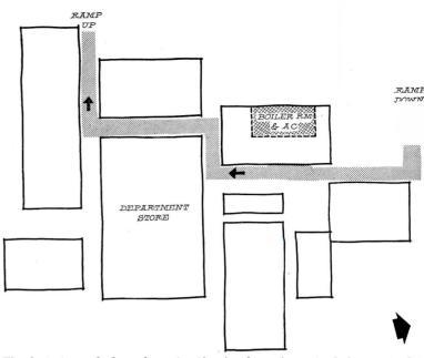
The first stage of planned construction involves nine out of the eventual 16 buildings. Underground it is all one building; the truck tunnel along the major axis serves as pipe chase for hot and cold water mains
