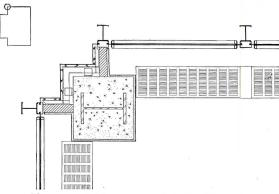
Above: outside corner detail. Glass is glare reducing pink which appears without color from inside. Bronze mullions were extruded from 7½ in. diameter tubes which are 2½ in. larger than the former maximum diameter available. Bronze covering columns was fabricated in long narrow extrusions fitted together. Extrusions were used because they wave less than plates.
