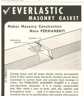
sensitive adhesive for use between sill and coping stones, brick and stone wall panels, and other places where
