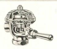
Self-cleansing by-pass guards against dirt or sediment in water. Thoroughly cleans by-pass orifice each time flush valve is actuated.
