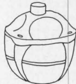
DRIVER UNITS ARE USED WITH HORNS. LINE MATCHING TRANSFORMERS ARE OFTEN BUILT IN.
