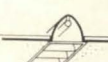
M—1-lamp recessed deep parabolic troffer with aluminum cross louvers 6 in. o-c. This type of fixture is suitable for installation at close spacing only and is so considered in the chart
