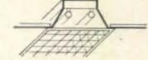
G—2-lamp recessed troffer, 2 ft x 4 ft, with egg-crate louver for 35° x 35° shielding
