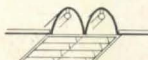
I—two type M fixtures side by side, forming 2 ft x 4 ft, 2-lamp recessed double parabolic troffer
