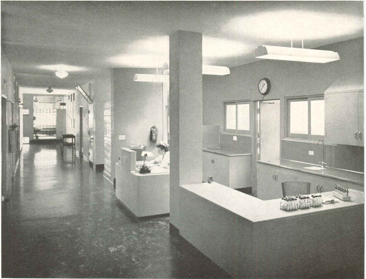
Nurses' stations are compactly surrounded by necessary floor services such as utility and sputum disposal rooms, janitor's closets; change in wall color at station reminds staff of entrance to sterile area. Cane fiberboard insulation on corridor ceilings keeps noise out of wards despite ventilation space above partitions
