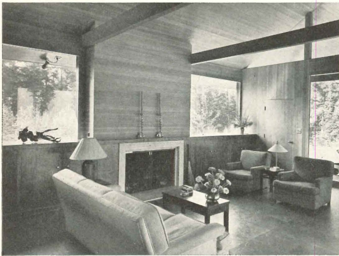
While some of the interiors are of plaster, this house shows its Northwest heritage with extensive use of wood — sloped ceiling of long hemlock boards, birch for cabinets and screens. Exterior of resawn vertical T & G Western Red Cedar
