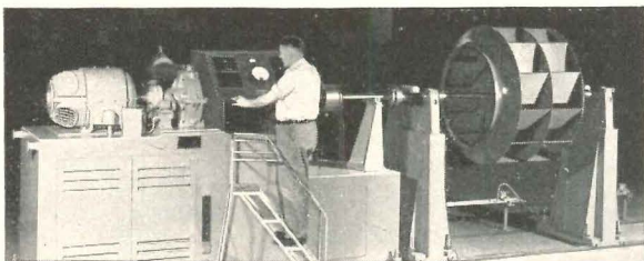
Special machines, built for TRANE (left), balance large fans both statically and dynamically. Above is a balancer for smaller size wheels.
