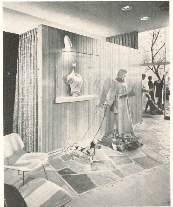
The architect designed all showcases and fixtures, cantilevering most of the wall cases. Flagstone floor of arcade is carried into interior and repeated in rear of shop which connects with Accessory Shop (next page)
