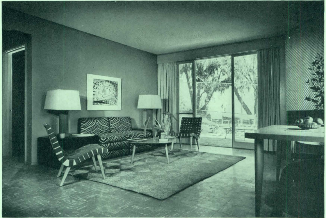
Ceilings of all units are pale yellow for reflective light, floors are gray asphalt tile to minimize upkeep. Fireplace hood is stamped aluminum
