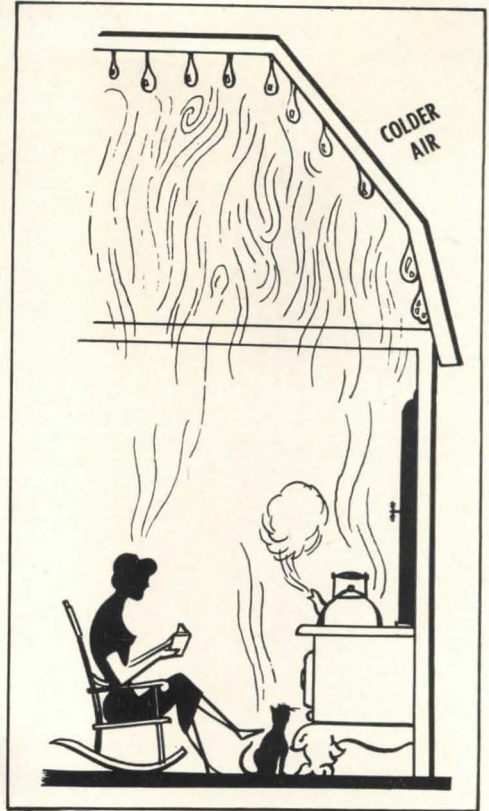
Condensation forms when the capacity of an air space at a given temperature is too small for the amount of vapor present.
