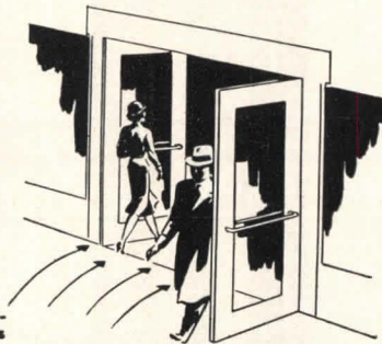
Another spring and hydraulic check controls outswing
