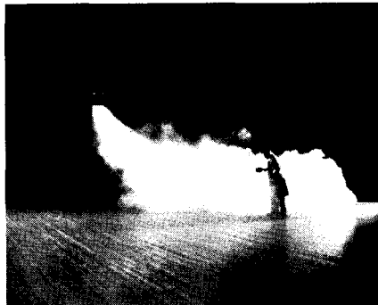
Adjustable diffusers for horizontal (top left) and vertical projection heaters (below left) give wide variety of diffusion patterns. Smoke is used in tests to check air currents
