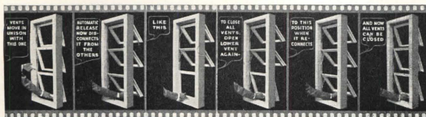
Operation of Dalmo Automatic Multiple Awning Type Window
