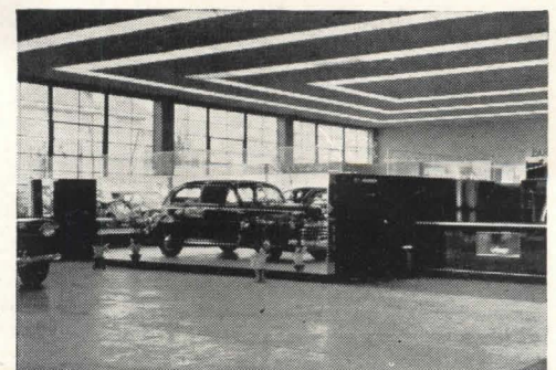
A FEELING OF SPACIOUSNESS is achieved in the showroom, and the display appears to be doubled by the use of plate glass mirrors on the end wall. In addition, Vitrolite is used here for attractive facing on the counter. Note the recessed ceiling lighting through panels of Reglex patterned glass.
