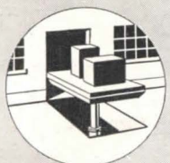
Levelator lowered becomes part of floor and can be trucked over. When loaded, Levelator rises smoothly to required level.
