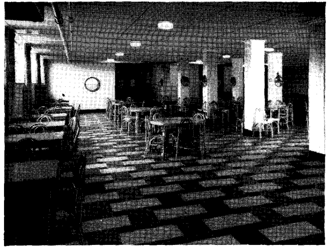
Asphalt tile presents many opportunities for colorful floors in cafeterias, kitchens, and other rooms located in basements or on grade level areas. Greaseproof asphalt tile is recommended for these floors as it is not harmed by spilled foods, greases, and other organic solvents.
