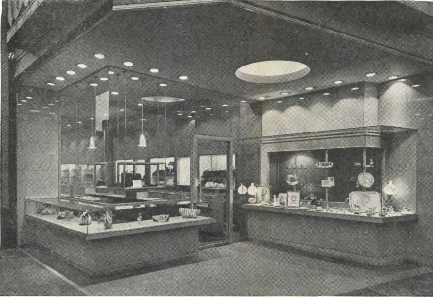
Above: behind plate glass, to left of door, and above outside showcase are two hanging cases for special displays, illuminated by "bullet-type" spots. Right: Silverware Department; hassock type chairs (designed by the architect) are finished in delft blue leather
