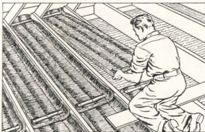
Simple method by which Double Thick KIMSUL, 16" wide blanket, was applied between ceiling joists in the attics of the 23 Bolling Square buildings. This illustration is from Page 6 of the KIMSUL Application Data File, a useful insulation manual, free on request to architects and builders.
