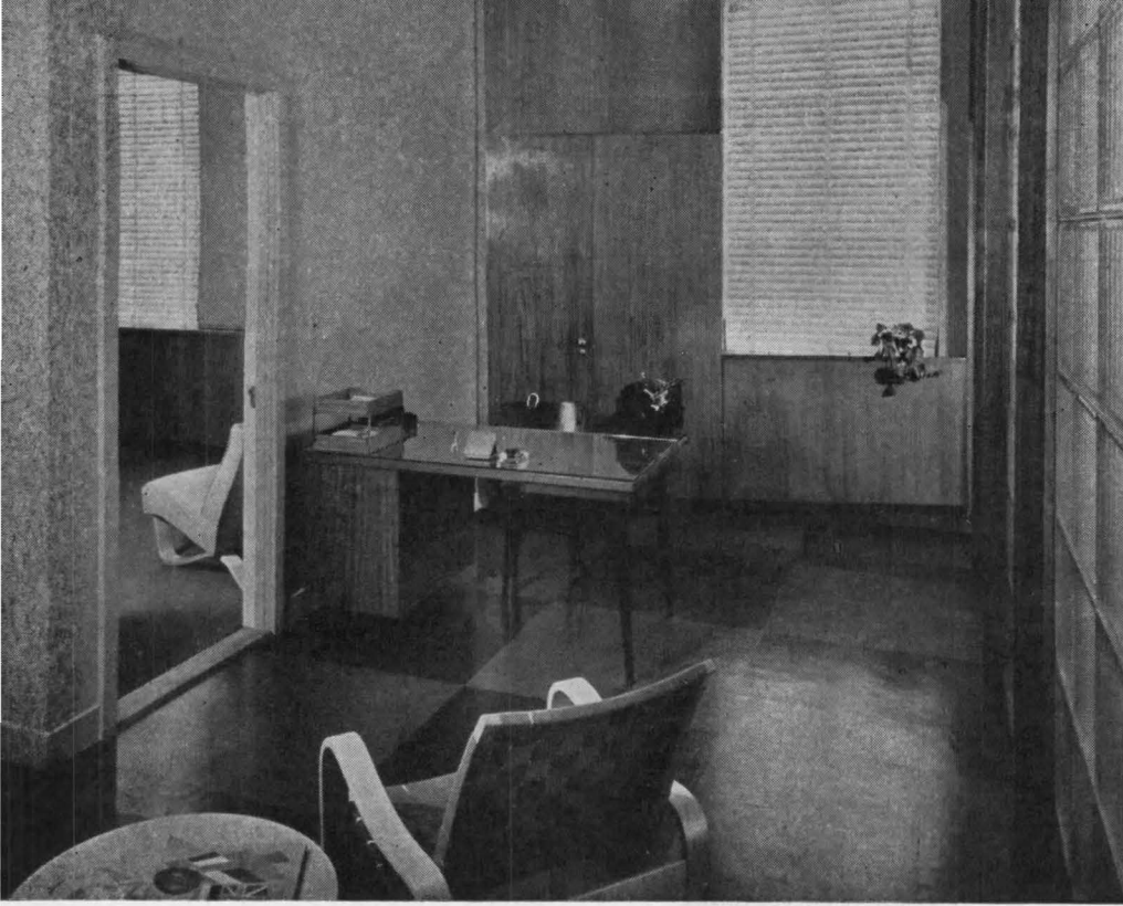
Angled coat closet and cabinets disguise a column in an office for a secretary
