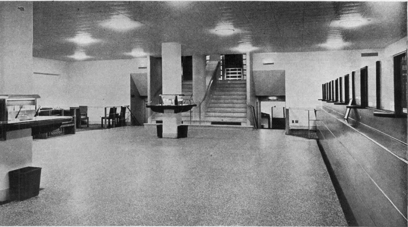
Above, full-width completed lower floor; below, the original half-plan. Note low ceilings, permissible here, in contrast to dignified height of main banking room above. Light-toned floor and walls reflect light. Fixtures "spill" enough across ceiling
