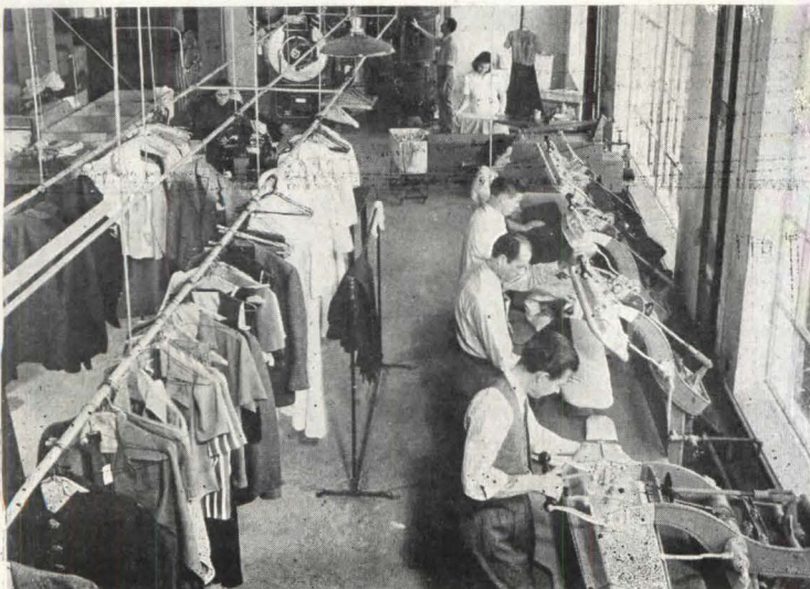
Dry cleaning arrangement in this laundry has been planned for the operators' ease, ample room has been allowed for both pressing operations as well as for handling of finished work
