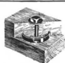
The TECO Ring Connector spreads the load on a timber joint over practically the entire cross-section of the wood.
