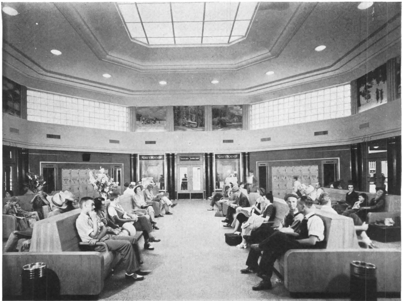
Above: Natural light enters the waiting room through a skylight and clerestory windows. Telephone booths and parcel lockers are made integral parts of the interior design.
