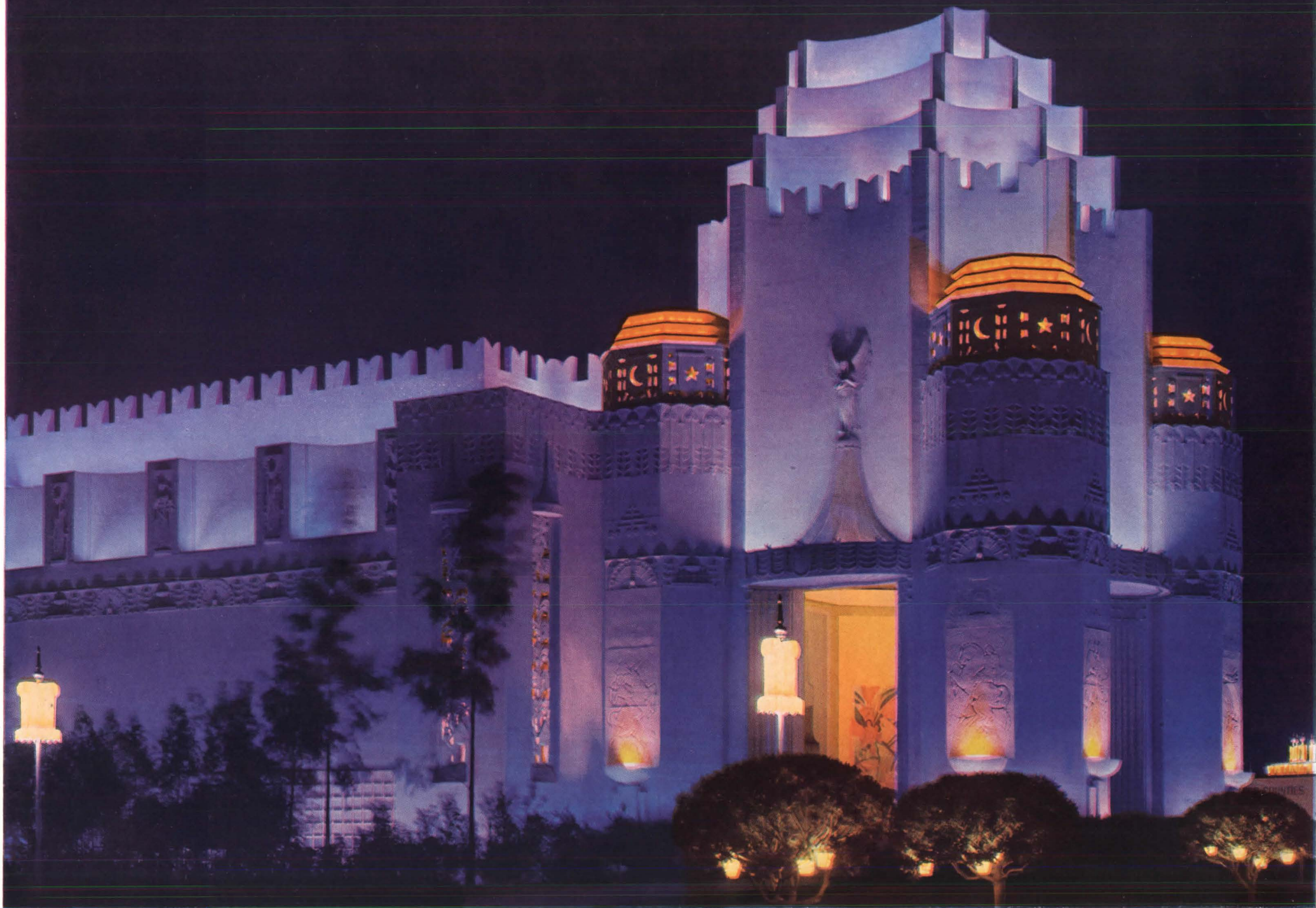
PLATE 9. Illumination of this Court is subdued, employing cool colors and low intensities. The main walls are carried in blue with a lavender overlay, while the set-backs are in blue; a mottled pink-and blue effect is used on the towers. All relief lighting—in grilles, niches, and louvers—is carried in amber to lighten the effect and tie it in with that of the other Courts.
