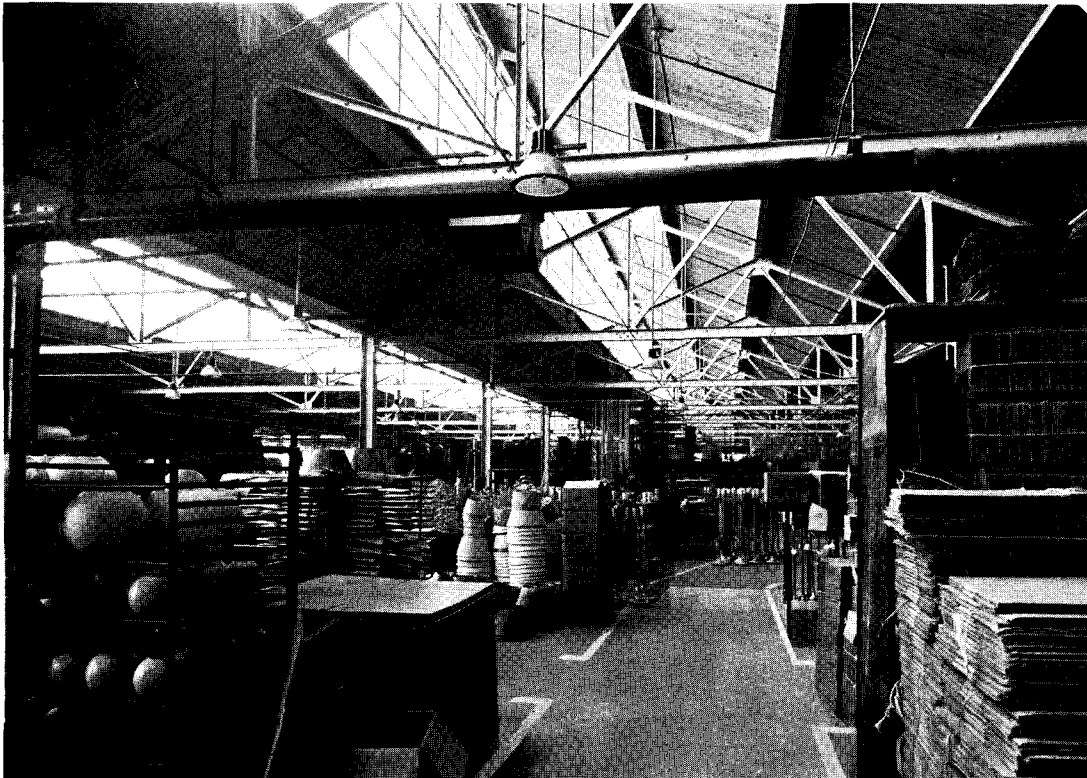
Interior, looking toward Assembly and Wiring Department. In left foreground is portable rack for conveying parts from one operation to another. Unit heaters are suspended. Lighting fixtures are direct type with prismatic reflectors.
