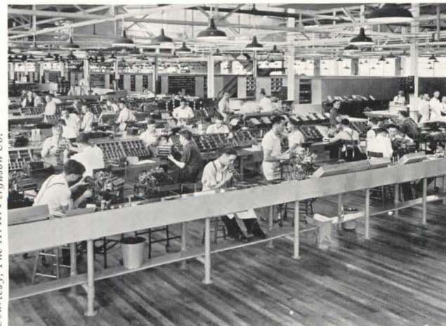
In this assembly plant the product—a calculating machine—is itself movable. Small parts are trucked to operators in boxes. The product is easily moved by hand through a series of assembly operations.
