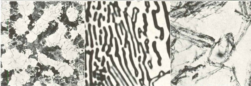
Researcher at metallographic microscope. Below, typical microphotographs (l. to r.): steel at 100 and 5,000 magnifications; filler for plastic, 175 magnifications.
