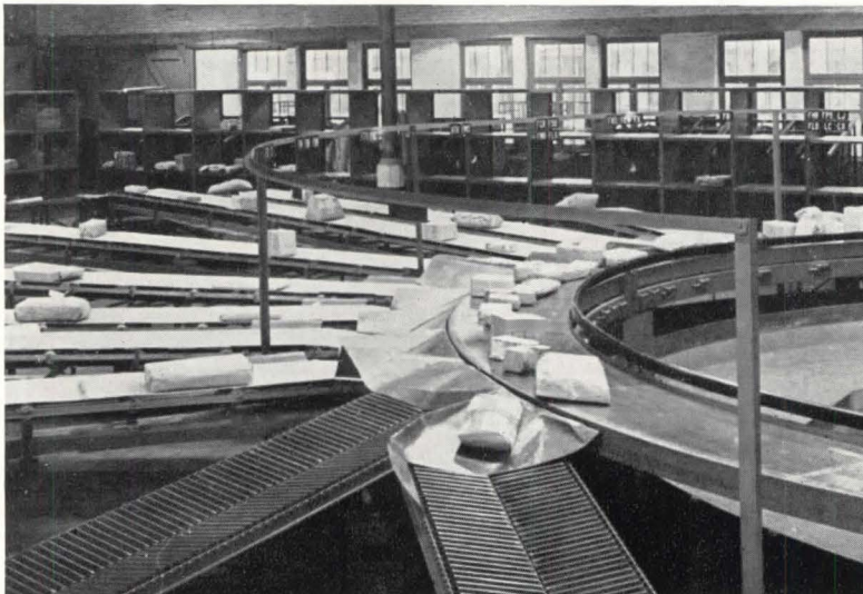
2. . . which carries them to central distributing ring where clerks sort them onto radial conveyers.
