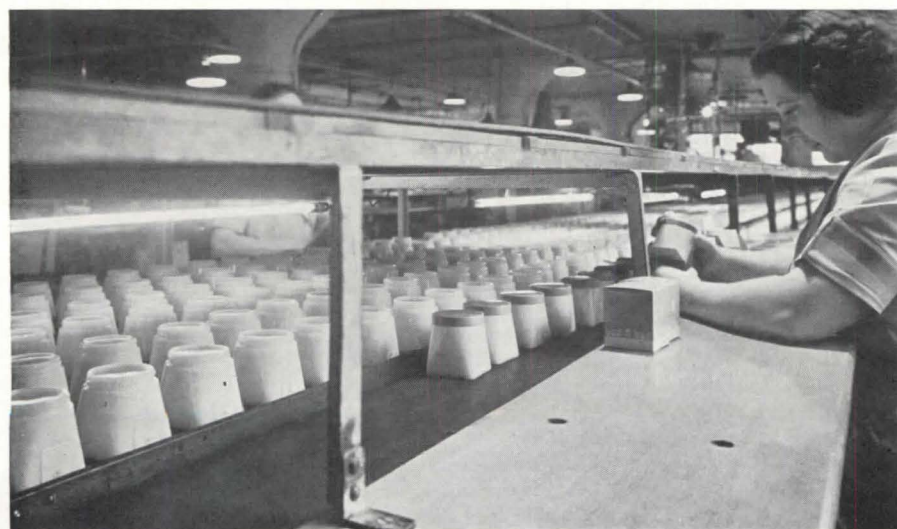
INDUSTRY: In this cosmetic factory, jars are passed under a bank of Sterilamps for sterilization while cooling.
