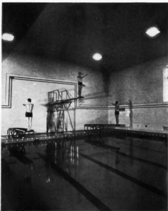
Diving apparatus in the practice pool. Frames may be detached at the floor leaving the deck unobstructed.
