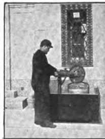
Raising filled can without leaving sidewalk. Can weighs 200 lbs. Pressure exerted only 14 lbs.
