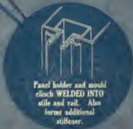
Panel moulding made separately and permanently SNAPPED INTO PLACE--NO SCREWS.
